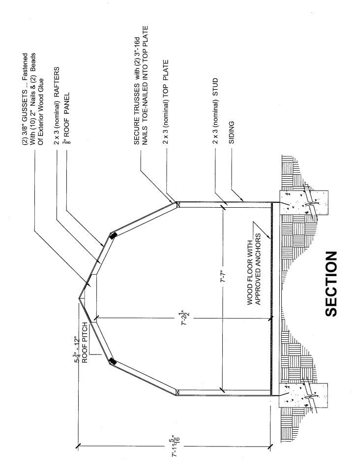
The equivalent ground snow load per ANCE 7-97 is 68 PSF which exceeds the 16.2 PSF pressure for a NOTES: 1) The Roof System of this 8 ft. wide Gabrel style building has a live load capacity of 35 PSF. 110 mph wind per ASCE 7-97.
